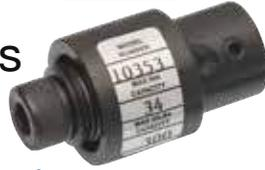
Rundown fixtures assist in testing the output of pulse, stall and clutch power tools. Neither our testers nor our rundown fixtures are designed or suited for impact tools.
