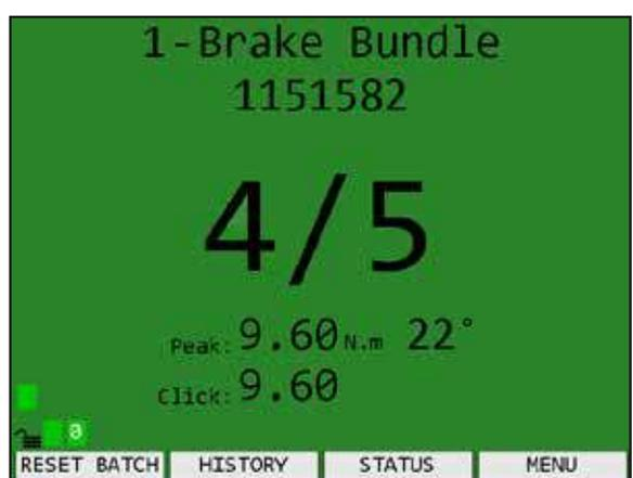
*In this application the operator stopped pulling when the wrench clicked. The fastener was not over-torqued, and this correct torque operation is displayed and tracked here.*
